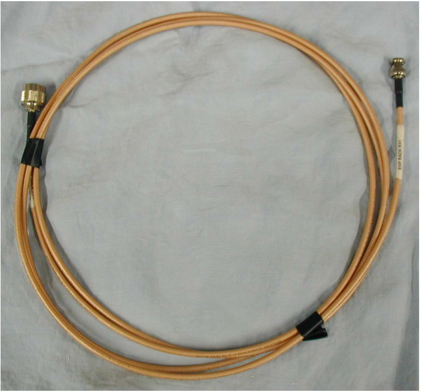
Figure 2, VNA test cable.
